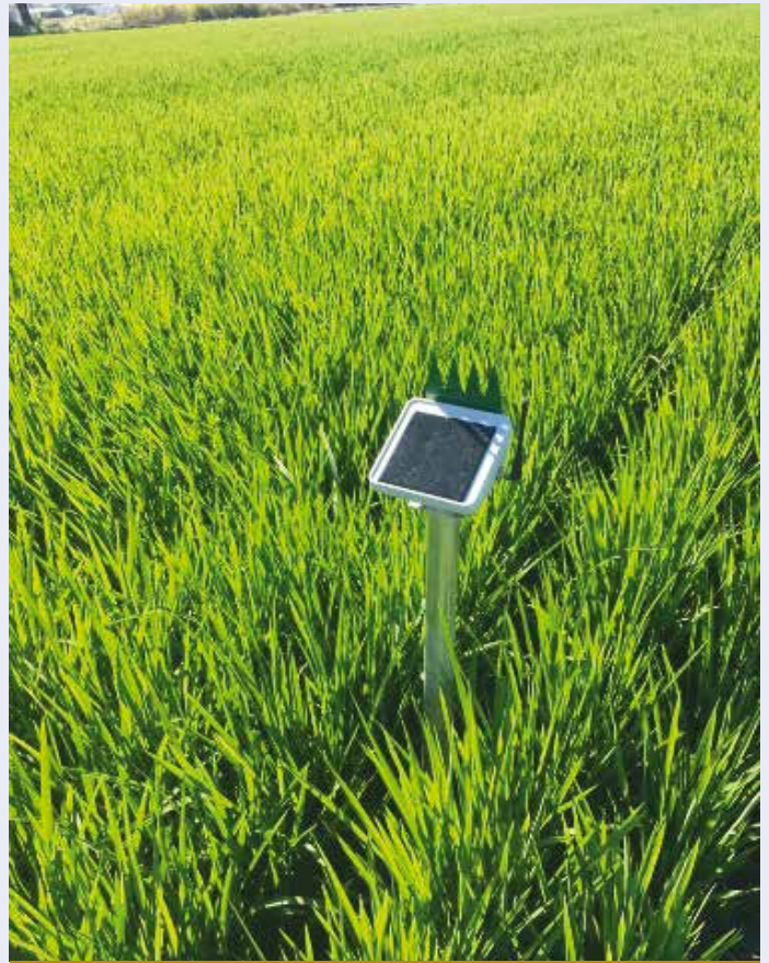
IMAGE 4: Sensor Pro capable of sensing water height and soil moisture.
