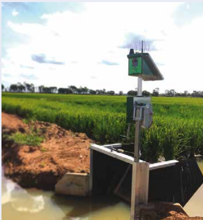
IMAGE 3: Padman Seasonal Autowinch and portable rubber inserts used in the automation of aerobic rice at De Bortoli Wines.
