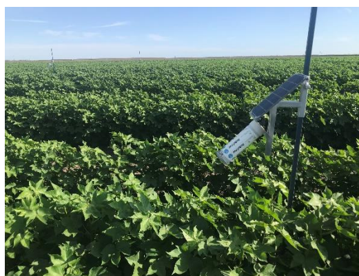
Figure 3: Infrared canopy temperature sensor monitoring crop stress in an irrigated cotton field
