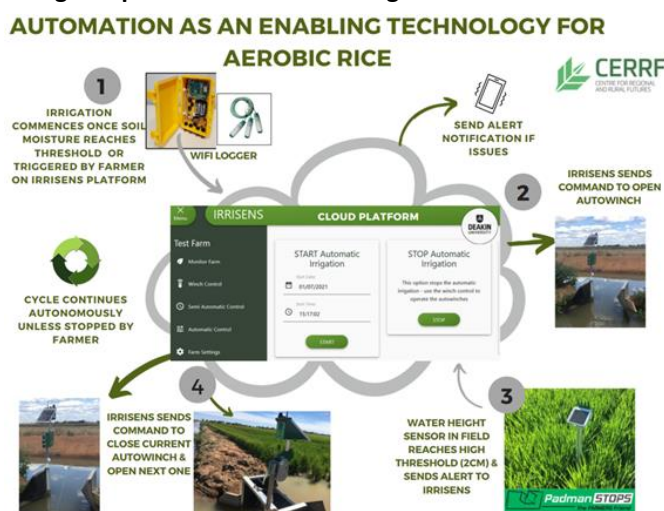
Figure 1: Diagram showing components of smart sensing and automation in aerobic rice
